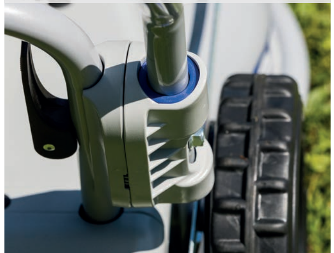
03. CENTRALIZED MOWING HEIGHT ADJUSTMENT
